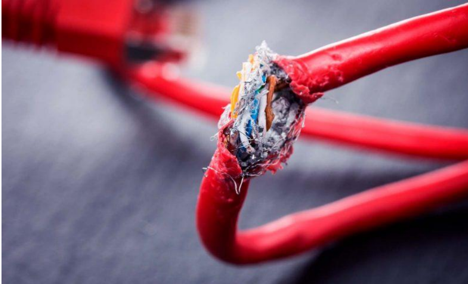
Figure2. 5 damaged distribution cable
