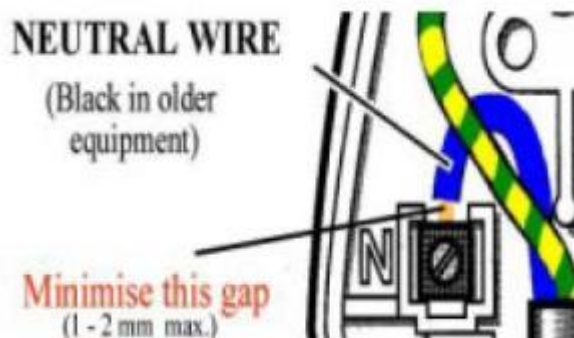
Figure 3. 3 gap between screw and insulation of
