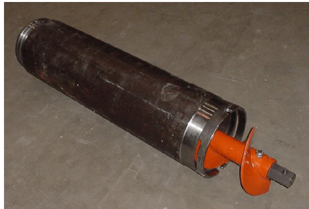
Figure 6. 3: Casing and auger assembly
