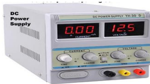
Figure 1-6 Power Supply - Variables:
